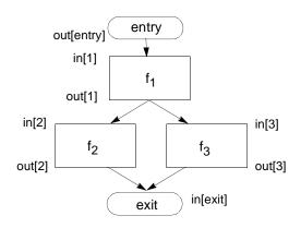
· Join node: a node with multiple predecessors
